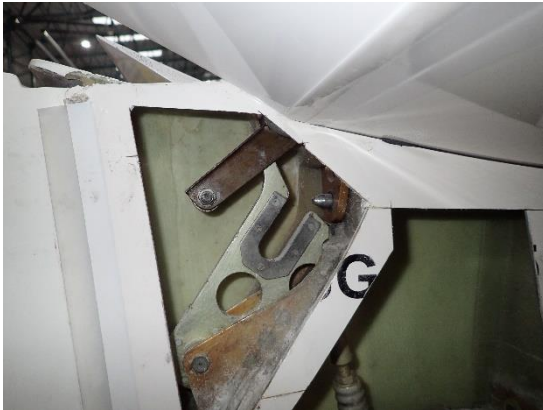
Disconnected elevator control
